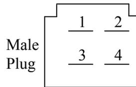
**Vehicle Wiring:** Connect to 4 Pin Plug supplied in kit.
